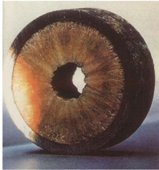
Figure 2.2. Wax deposit reducing the effective diameter in a retrieved pipeline (Singh et al. , 2000).
