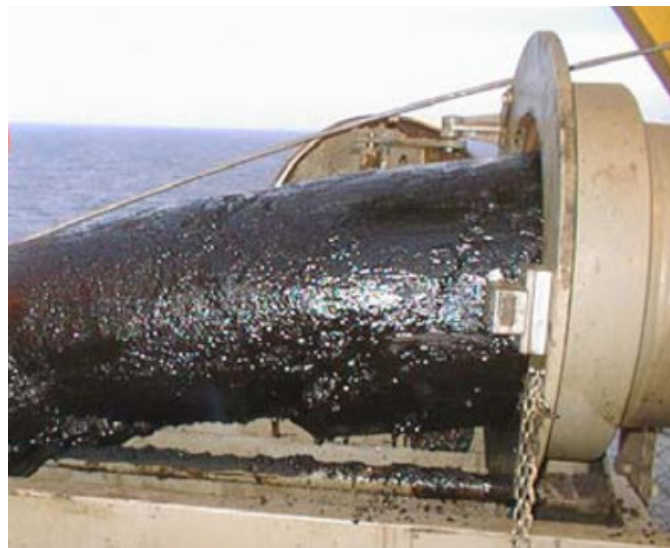
Figure 2.3. Outcome of the pigging process for gelled waxy crude (Hydrafact, 2014).
