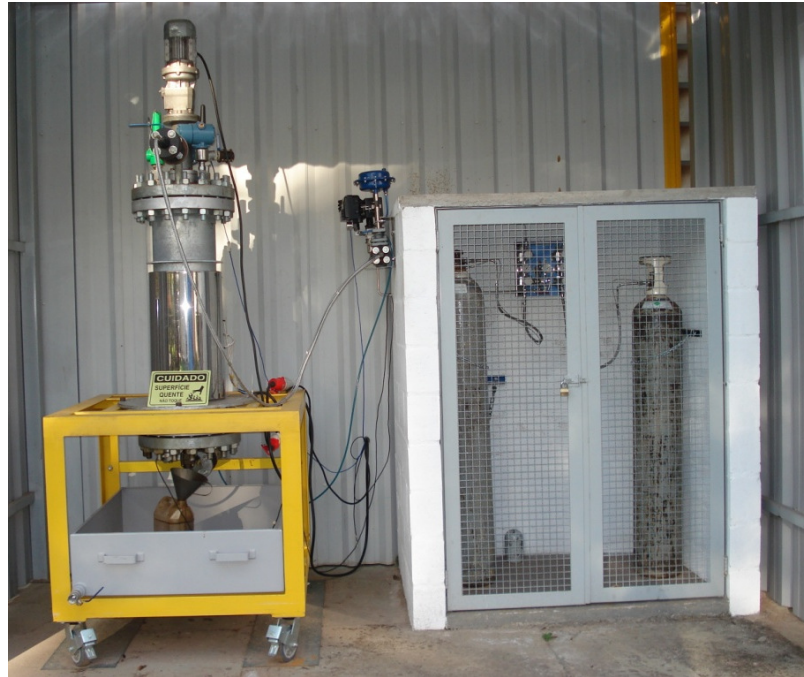
Figure 3.7. Pressurization system (Luthi, 2013).
