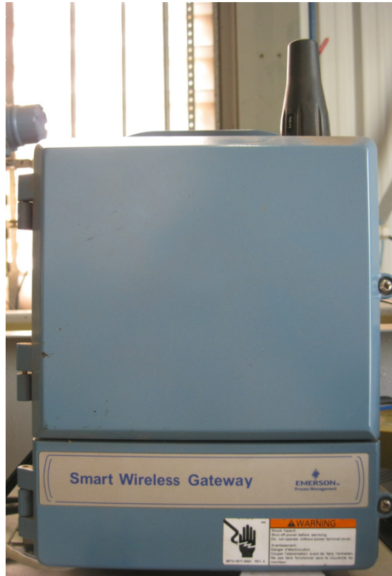
Figure 3.8. Gateway used for receiveing the data from the wireless sensors.
