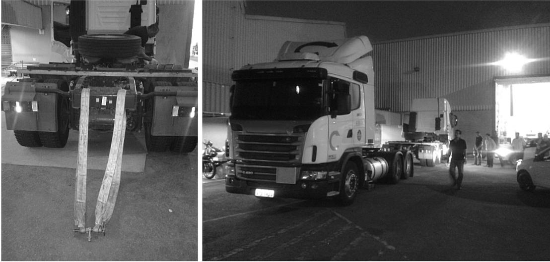
Figure 2.5: *Left*: Band used to pull vehicle.
