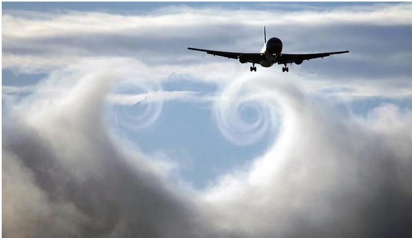
Figure 4.1: Vortical structures formed by aerodynamic wake from wing tip and flap.
