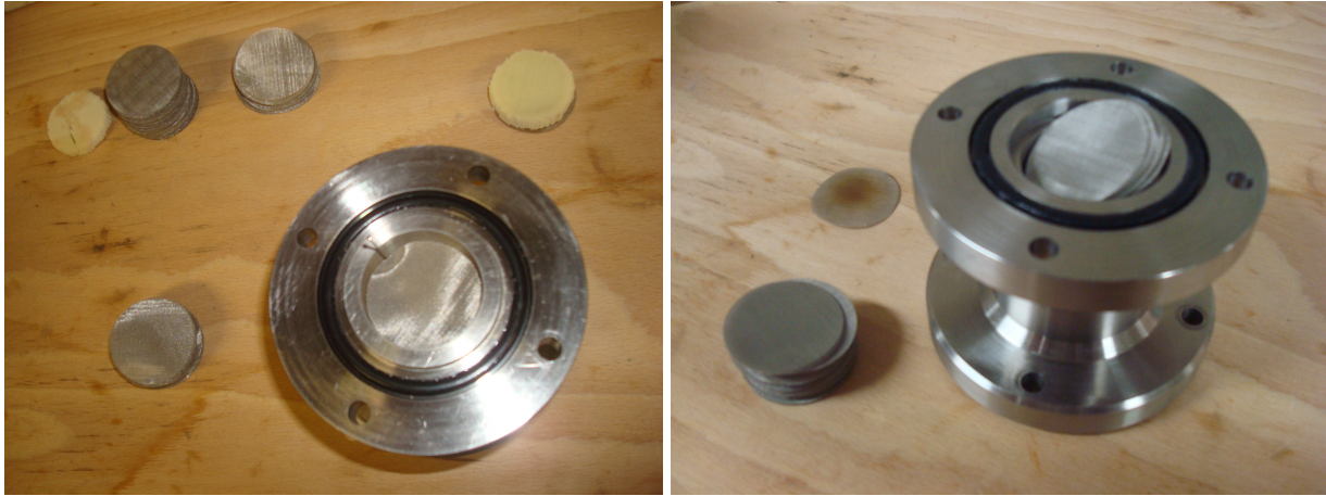
Figure 3.6: Stainless Steel Grids, ceramic washers and stack/regenerator holder.
