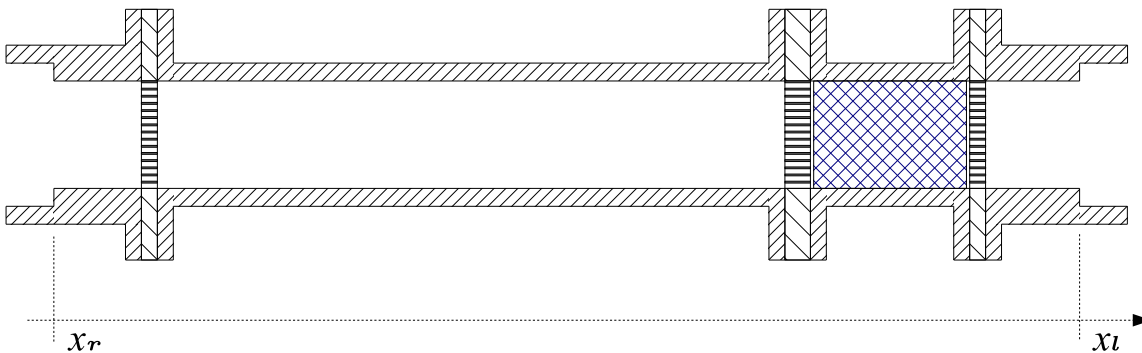
Figure 3.10: Sketch of the inverted ThermoAcoustic Core.
