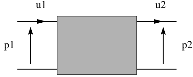
Figure 2.2: Adopted pressure-volume velocity convention for the quadripole description; anti-symmetric orientation.
