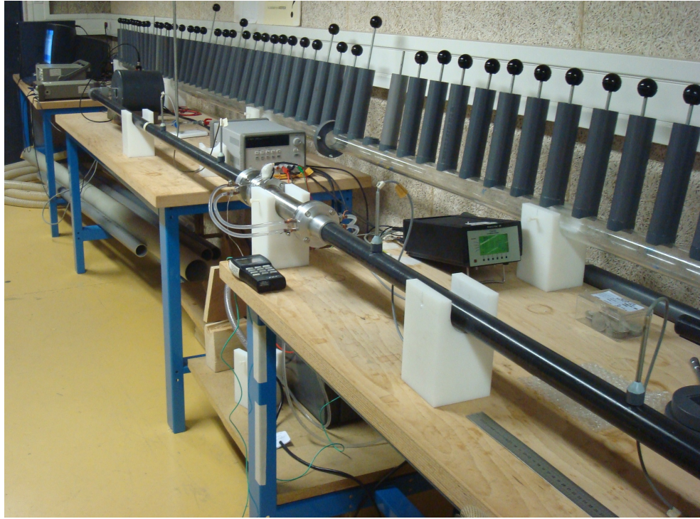
Figure 3.4: Experimental setup - Two-Load Method.
