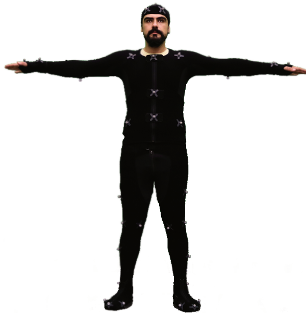
Figure 2.5: Motion capture performer in the T-Pose with the Vicon Shōgun™ standard 53 marker setup.
