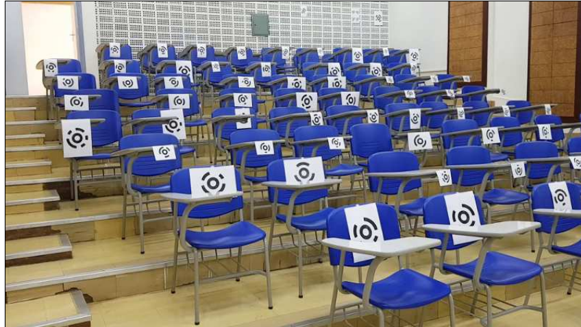
Figure 31 – One of the entire class detection experiments, to evaluate the overall performance and the effect of the scanning procedure. In this setup, the scanning occurred from the class floor, starting scanning on the left and walking to the right.
