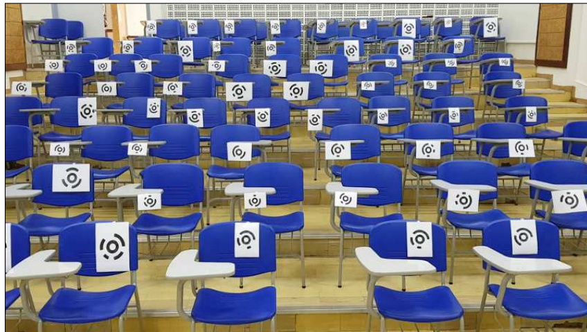
Figure 32 – Another setup for the entire class detection experiment: in this one the scan started from the professor's stage, starting scanning from the center of the classroom.
