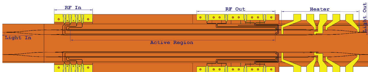
Figure 3.1: LX8242 DP-QPSK TFPS modulator by Gigoptix/BrPhotonics schematic. Upper gold trace is shown in yellow, while bottom plane metalization is orange. Optical waveguide trench is shown in blue.
