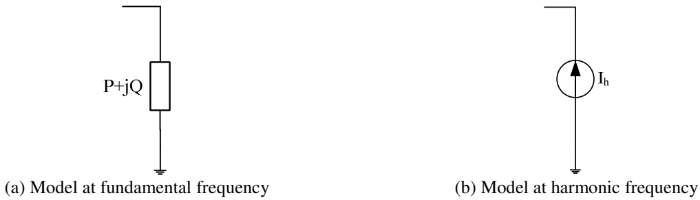
Figure 2.5: Model for nonlinear appliances.
