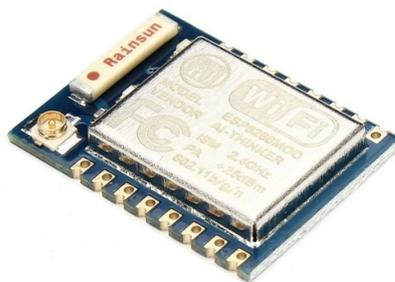
Figura D.3: Módulo WiFi ESP8266 ESP-07.
