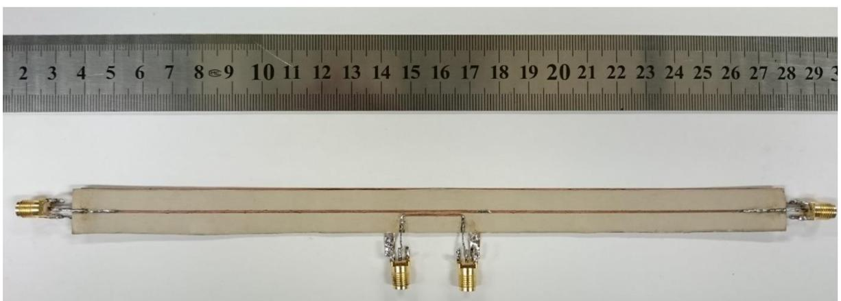
Figura 3.9: As microstrip coladas back-to-back com os conectores SMA.
