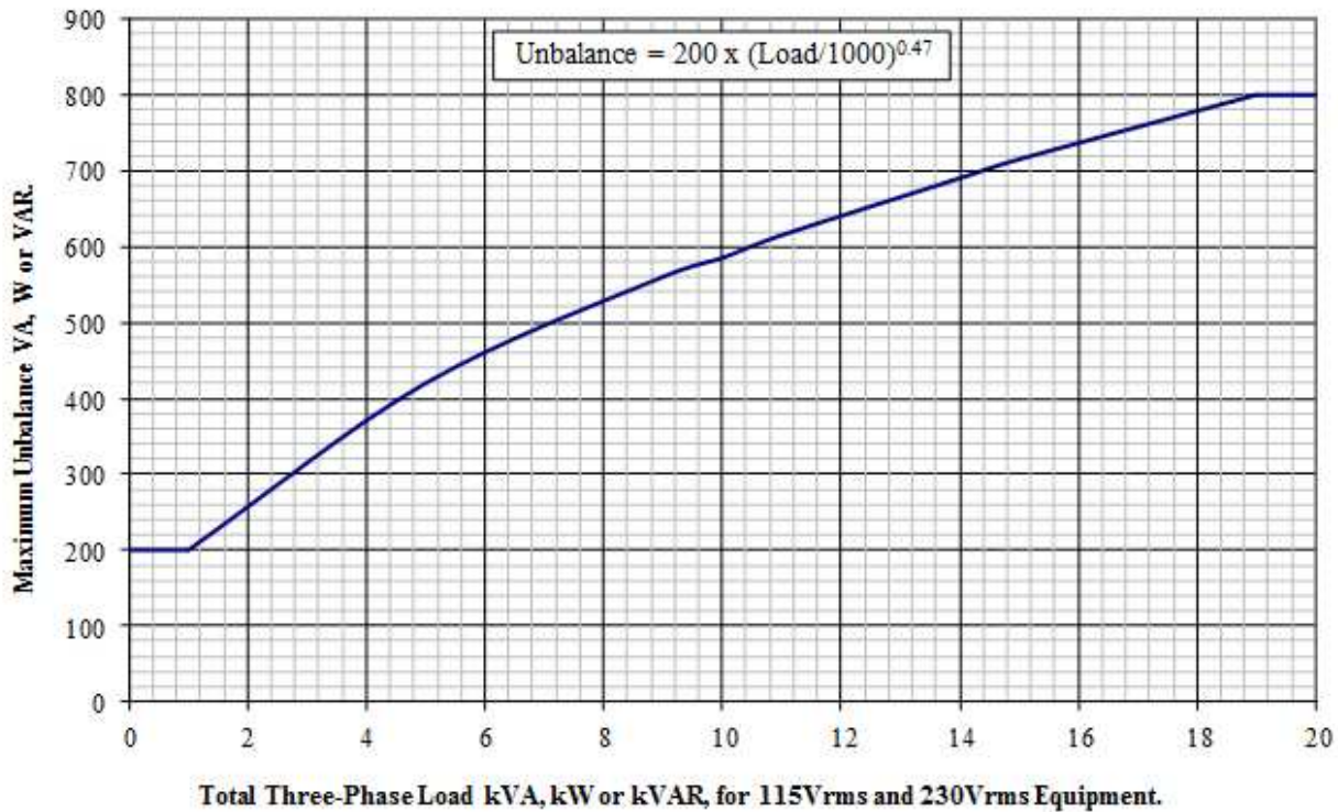
Figure 2-17: Allowable Phase Unbalance for Three Phase AC Loads [28]
