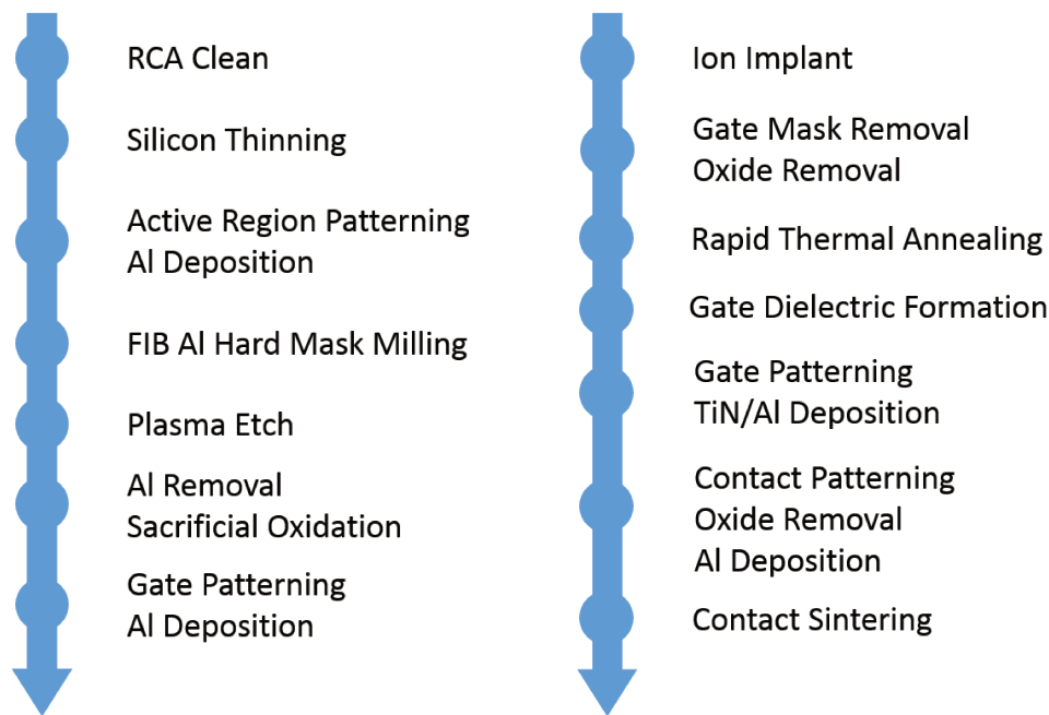
Figure 16 – Summarized process steps for FinFET fabrication
