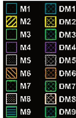
Figure 3.8 – Layer map identification for both routing and dummy metals.
