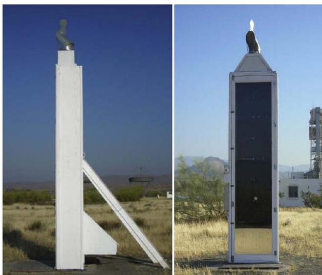
**Figura 7.2:** Vistas lateral e frontal da chaminé solar experimental (ARCE et al, 2009)
