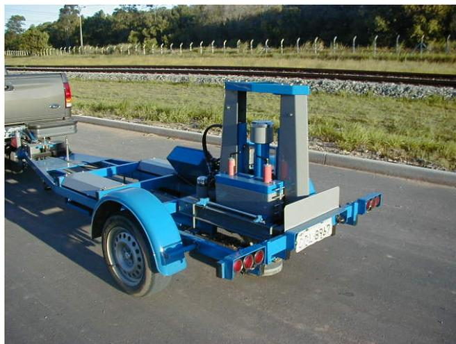
Foto 3.8 - *Falling Weight Deflectometer* - FWD
