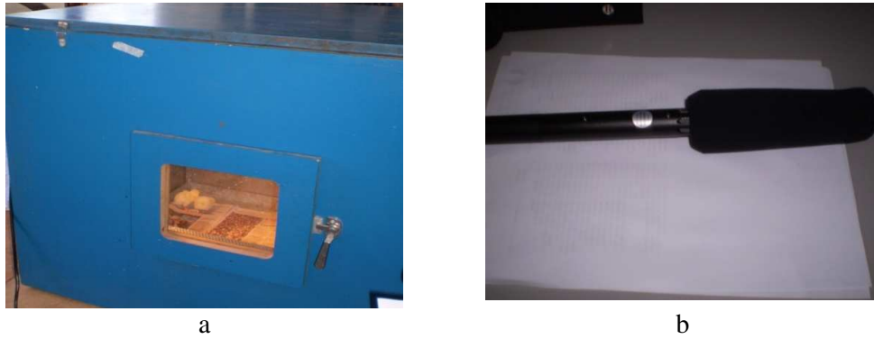
Figure 1. Semi anechoic chamber (a) where the chicks were placed and the sound recorded using a unidirectional microphone (b).
