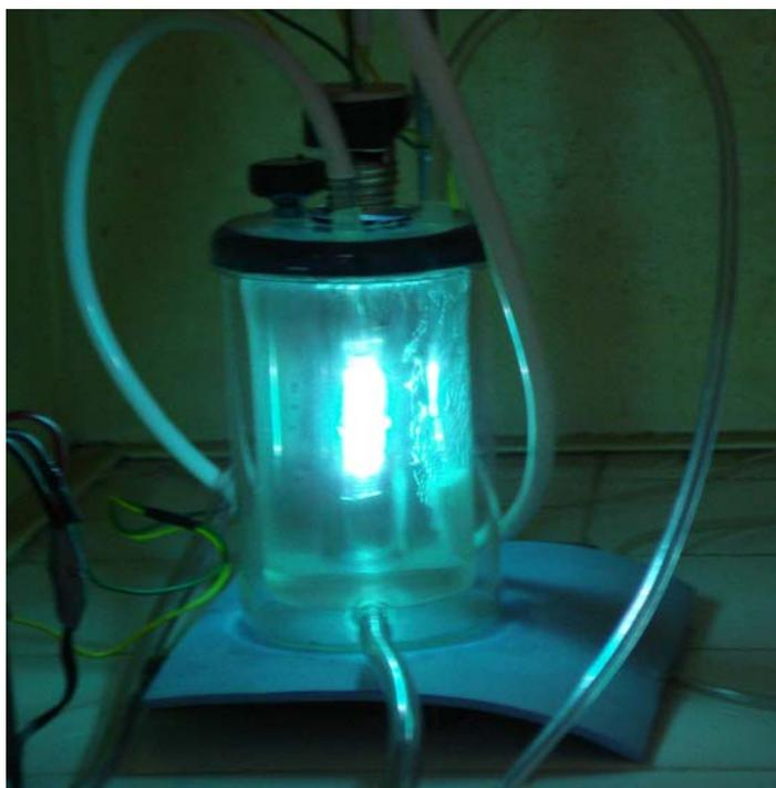
**Figura 7:** Reator de UV artificial.
