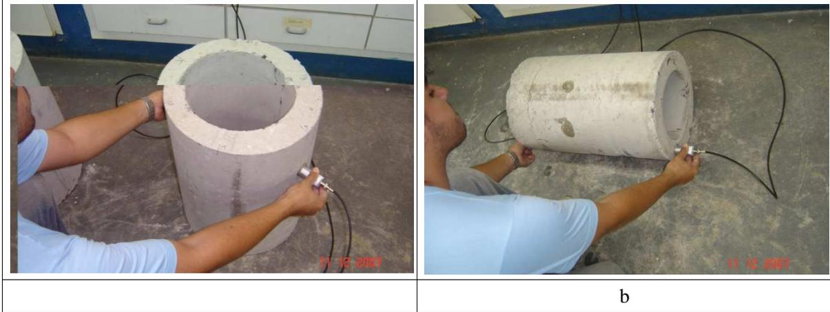
FIGURE 2. Radial measurement (a) and longitudinal measurement (b)
