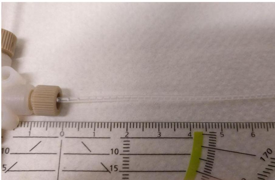
Figure 12 Image of the segmented flow at an oxygen liquid ratio of three to one at the beginning of the reactor.
