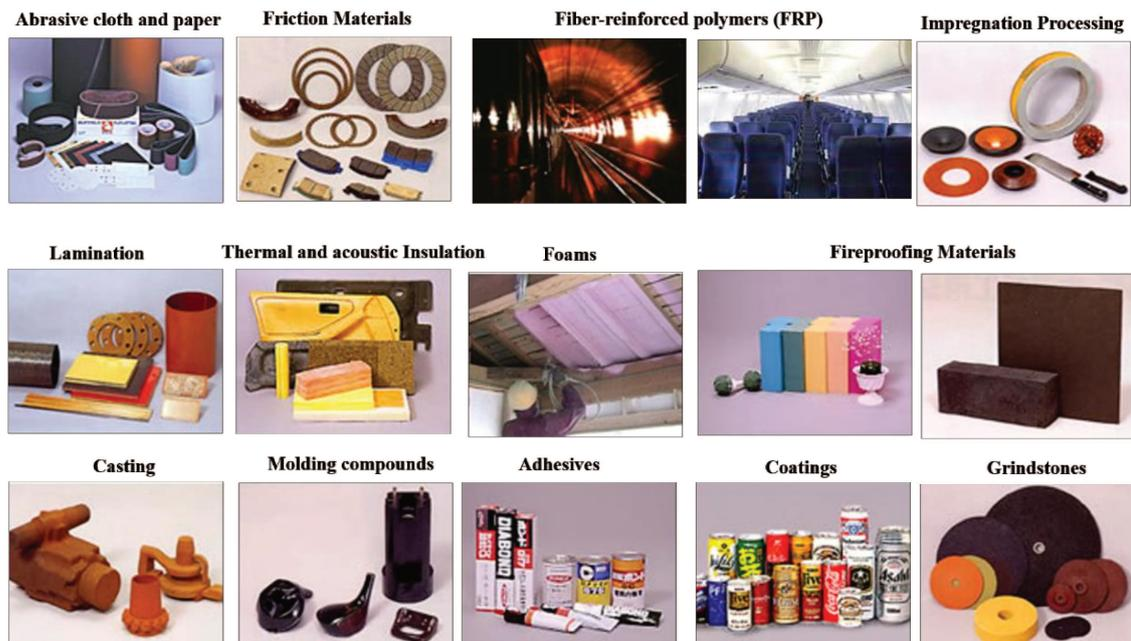
**Figure 2.15** - Phenolic resin applications (adapted from Showa Denko Group, 2017).
