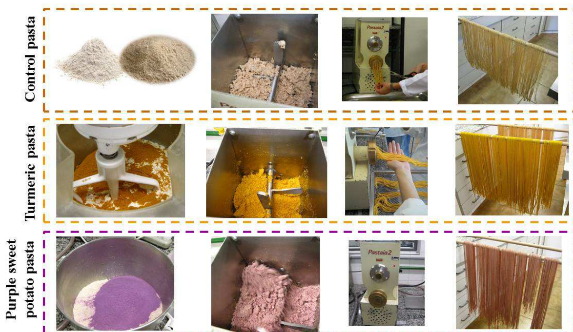
Figure 3. Processing of control, turmeric and purple sweet potato fresh whole wheat pastas
