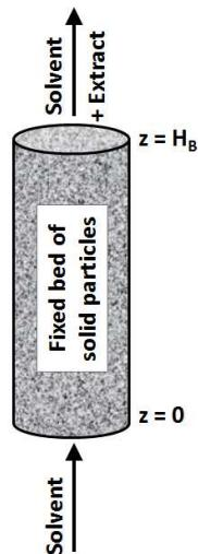
**Fig. 3.5** A typical fixed bed extractor of the SFE process ( $z$ : axial coordinate,  $H_B$ : bed height)
