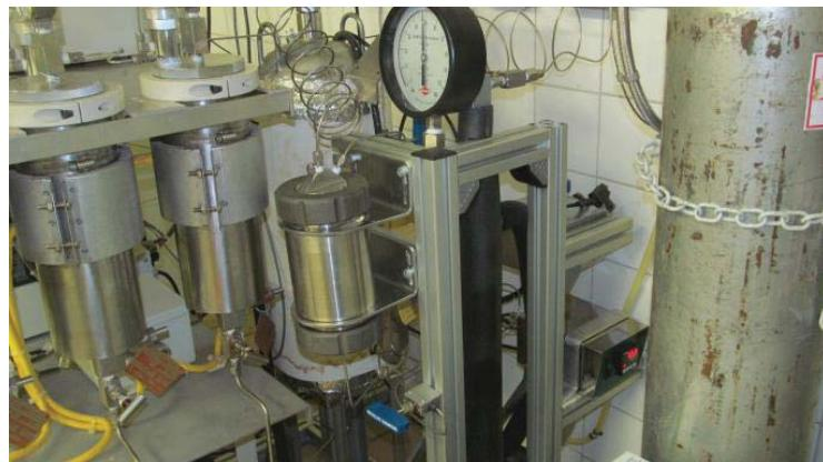
**Fig. (9).** Components of the homemade online subcritical adsorption-based device developed to allow effective CO<sub>2</sub> recycling.
