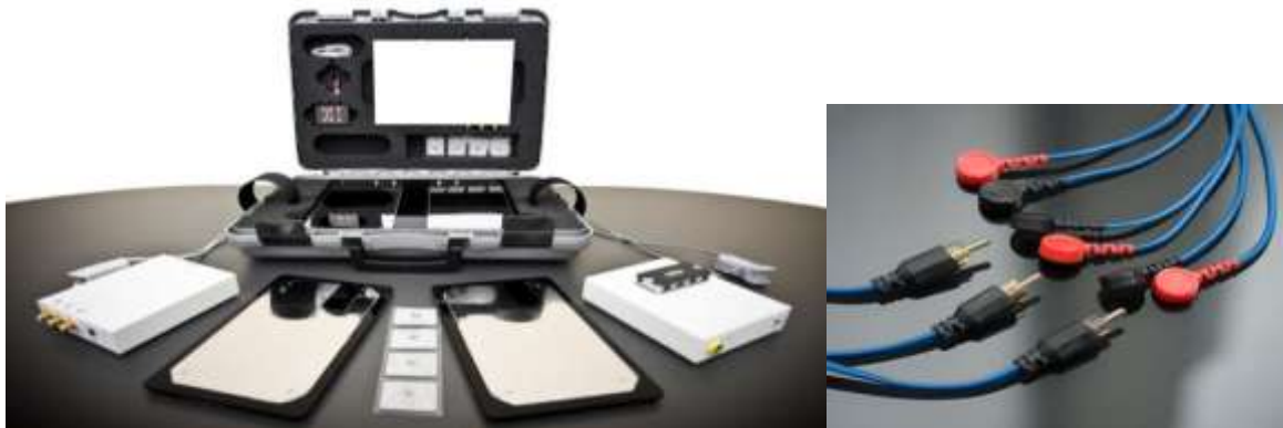
Figure 1A- Hardware within an interface box, disposable electrodes, reusable plates, reusable cables and software installed on a computer; Figure 1B - Reusable cables.
