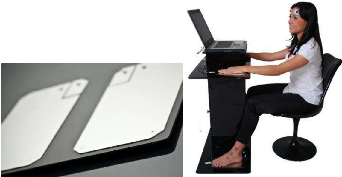
Figure 4A – Close of the stainless steel reusable plates and Figure 4B patient doing an examination with head electrode.
