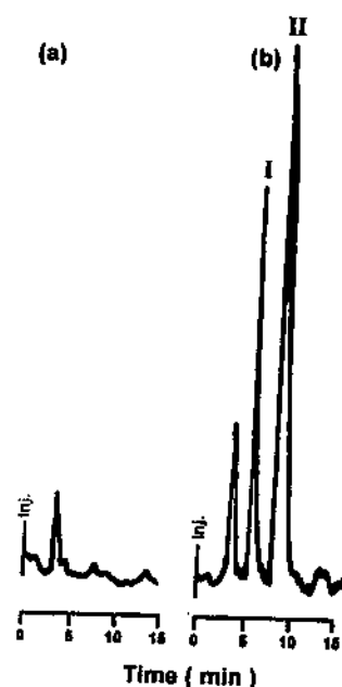
Fig. 1 Examples of obtained HPLC chromatograms. Panel (a): blank plasma showing the absence of peaks at the retention times of the compounds of interest, panel b: plasma sample withdrawn 6 hours after the administration of 50 mg of atenolol. Atenolol concentration measured in this sample was 170 ng/ml. Peak I: atenolol, peak II: metoprolol (internal standard).
