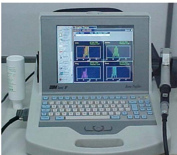
**Figura 2** – Aparelho *DBM Sonic<sup>®</sup> BP*
