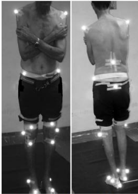
Figure. Typical configuration of the reflective markers.
