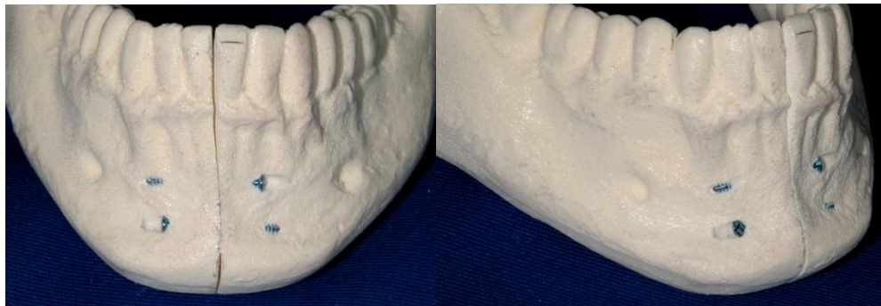
Figure 4: Fixation of LST group, lag screw technique, (a) front view, (b) side view.
