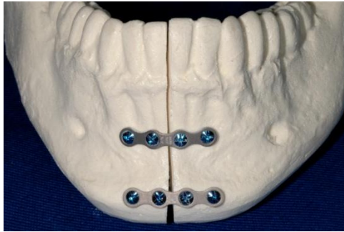
Figure 2: Fixation of 2PLL group, parallel miniplates, one in the tension zone and the other in the compression zone.
