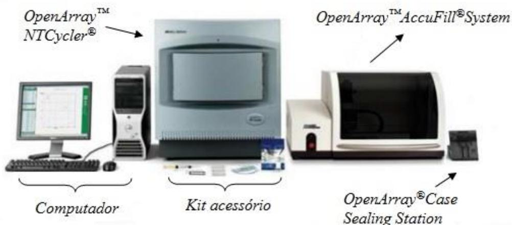
**Figura 5.** Plataforma *TaqMan® OpenArray™* (Applied BioSystems).
