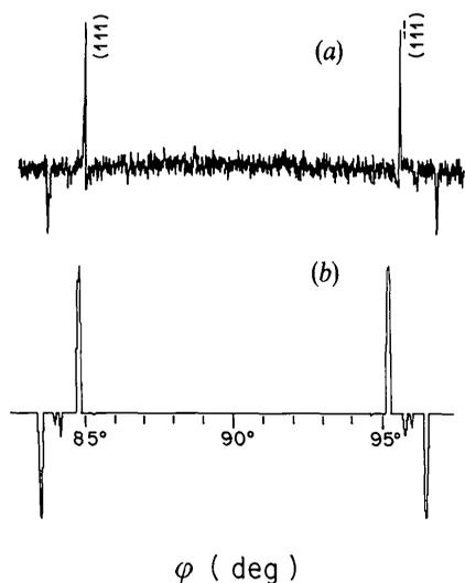
Fig. 4. Portion around  $\varphi = 90^\circ$  of the 002 GaSb Renninger scan using  $\text{Cu K}\alpha_1$ : (a) experimental and (b) simulated. The peak asymmetry indicative of the good quality of the crystal cannot be simulated, since the *MULTX* program only applies to mosaic crystals.
