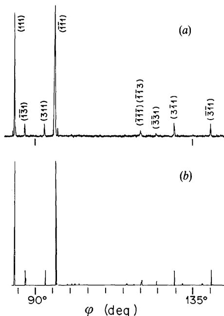
Fig. 5. 002 Renninger scans using  $\text{Cu K}\alpha_1$  applied to heteroepitaxial structures. (a) Experimental RS for a GaAs layer on top of an Si substrate and (b) the corresponding simulated RS.
