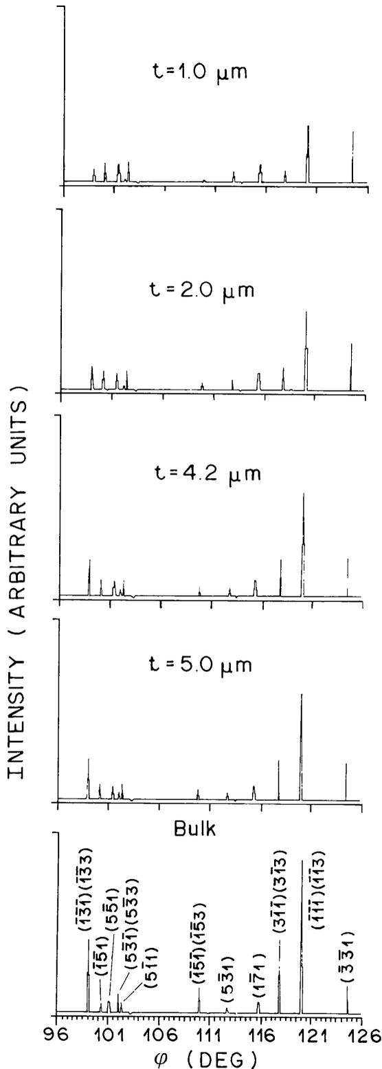
Fig. 2. Simulated 002 GaAs Renninger scans using  $\text{Cu } K\alpha_1$  for different layer thicknesses to show the influence of the diffracted-beam path lengths on the intensities in a RS. Bulk thickness: 350  $\mu\text{m}$ .
