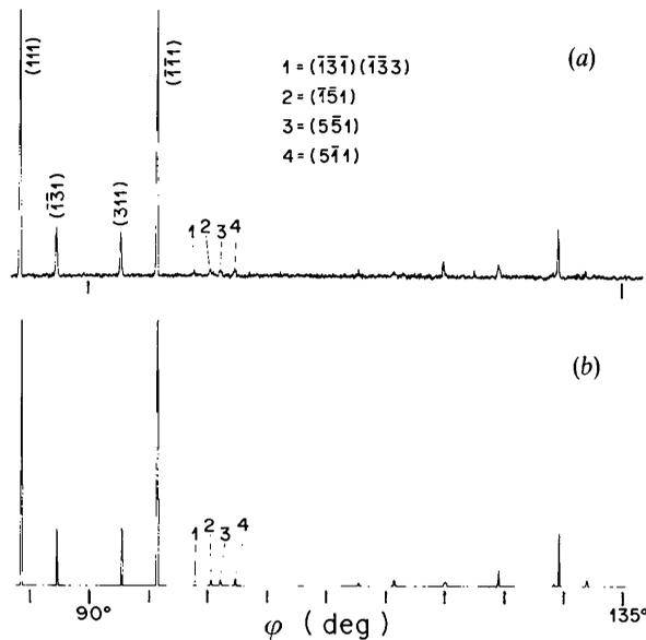
Fig. 6. 002 Renninger scan using  $\text{Cu } K\alpha_1$  applied to the  $\text{In}_x\text{Ga}_{1-x}\text{As}$  ternary layer with  $x = 0.035$ : (a) experimental and (b) simulated.
