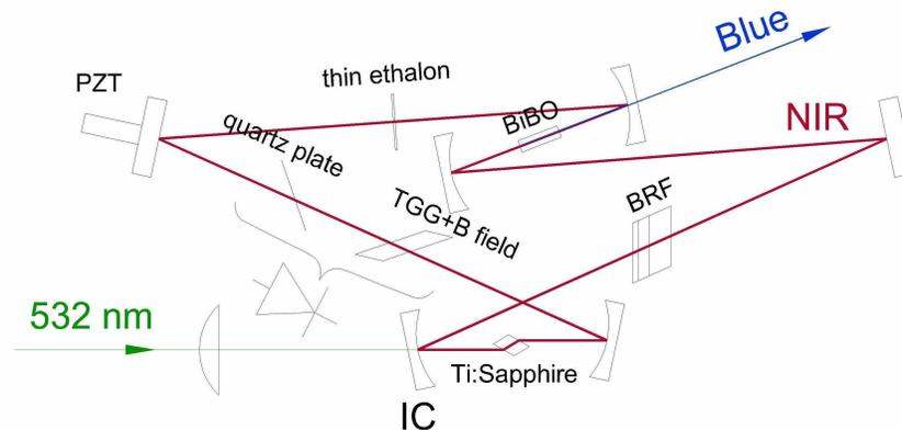
Fig. 2. Schematic diagram for intracavity second harmonic generation in another Ti:sapphire laser (total cavity length is 114 cm). Two fold mirrors (ROC=5 cm) were used to produce a tight waist at the BBO position. An optical diode and a thin coated etalon were introduced for single-frequency operation.
