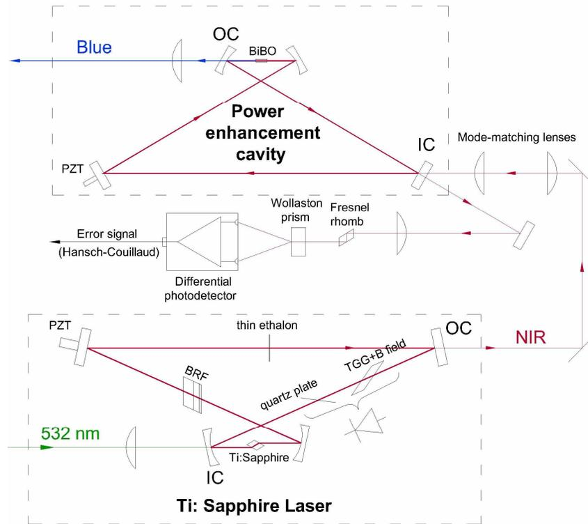
Fig. 1. Schematic diagram showing our single-frequency Ti:sapphire ring laser and its frequency doubling into an external cavity, locked by the Hänsch-Couillaud technique [8]. The Ti:sapphire laser and doubling cavity lengths are 104 and 62 cm.
