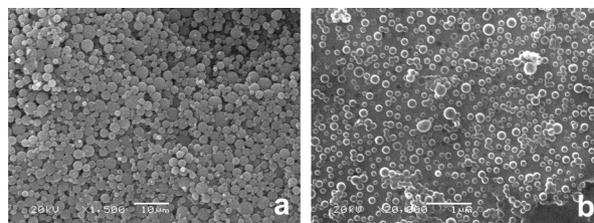
**Figure 1.** SEM images of: (a) microspheres and (b) nanospheres of InTPP-loaded PLGA prepared using an emulsion/evaporation method, employing PVA as an emulsifier, and with agitation rates of 1200 and 14,000 rpm, respectively.
