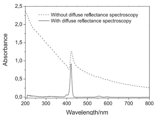
**Figure 5.** Absorbance spectra of an InTPP-loaded nanoparticle suspension in isobutyl alcohol at 27 °C obtained (—) with and (---) without the diffuse reflectance accessory. The total InTPP concentration in the suspension was  $2.0 \mu\text{mol L}^{-1}$ .
