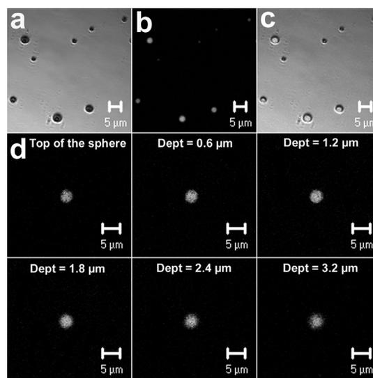
**Figure 3.** Confocal microscopic images of InTPP-loaded microspheres: (a) using differential interference contrast microscopy (DICM), (b) with excitation of InTPP using an argon laser, (c) overlapping of both former images, and (d) optical cross section taken from the top of the spheres (top row) with a gradual increase in depth of  $0.6 \mu\text{m}$ .
