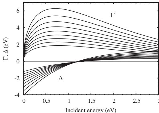
FIG. 2. Fixed-nuclei level shifts ( $\Delta$ ) and widths ( $\Gamma$ ) for the interatomic distances given in Sec. III A. The peak heights of  $\Gamma$  around  $0.70$  eV monotonically increase with the interatomic distance, while the level shift values at zero energy are monotonically decreasing (the latter trend is inverted at higher energies due to the crossings around  $1.2$  eV).
