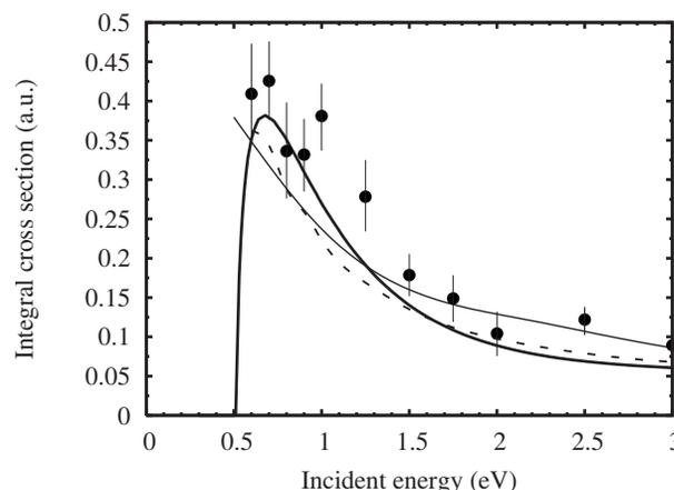
FIG. 4. Integral cross section for the  $0 \rightarrow 1$  vibrational excitation of  $H_2$  by positron impact. Thick solid line: present result; thin solid line: theory of Sur and Ghosh [81]; dashed line: theory of Gianturco and Mukherjee [24] (corrected results of Ref. [23]); circles: experimental data of Sullivan *et al.* [4].
