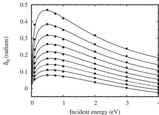
FIG. 1. Fixed-nuclei  $s$  wave scattering phase shifts ( $\delta_0$ ) for the interatomic distances given in Sec. III A (peak heights around  $0.50$  eV monotonically increase with the interatomic distance). The lines are least-squares fits to the SMC calculations (squares).
