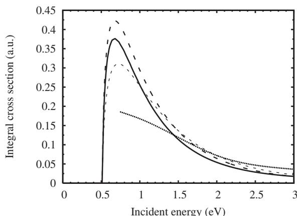
FIG. 3.  $S$  wave partial cross section for the  $0 \rightarrow 1$  vibrational excitation of  $H_2$  by positron impact. Dotted line: ANV result of Refs. [31,32]; thin dashed line: Condon approximation for the level shift; thick dashed line: local approximation for the level shift; solid line: full nonlocal calculation.
