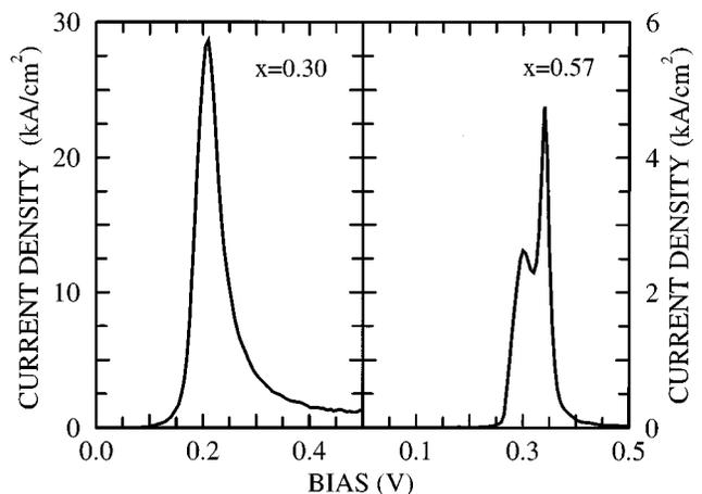
FIG. 4. Current density–voltage characteristics for the double barrier structure of Fig. 2(b).
