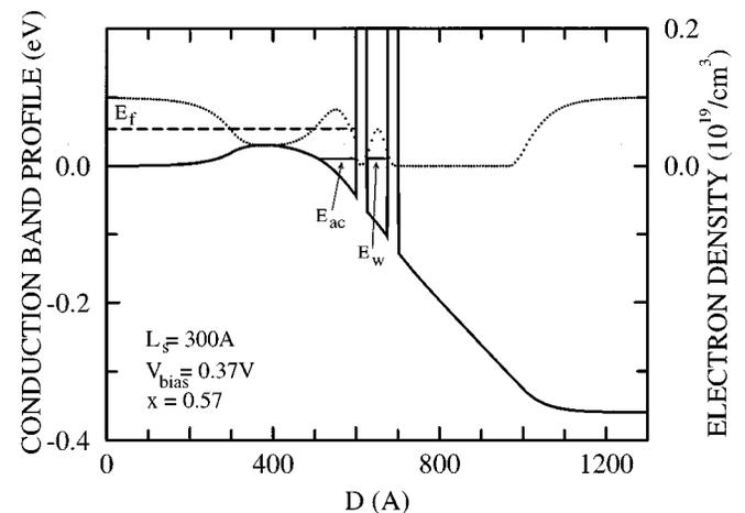
FIG. 1. Profile of the conduction band minimum and electronic density (dotted line) for a double barrier structure under applied bias. The quasibound states in the accumulation layer and the double barrier quantum well are also shown.
