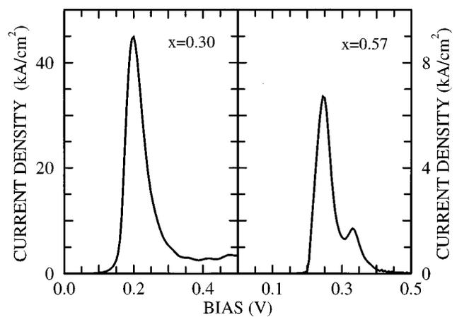
FIG. 3. Current density–voltage characteristics for the double barrier structure of Fig. 2(a).
