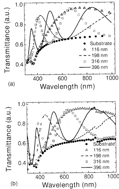
FIG. 3. Transmittance of the  $\text{SiO}_x\text{N}_y$  films as a function of wavelength for various thickness: (●) substrate; (△) 116 nm; (---) 198 nm; (□) 316 nm; and (—) 396 nm. (a) Simulated and (b) measured.
