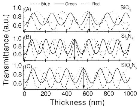
FIG. 4. Simulated transmittance spectra of (A)  $\text{SiO}_2$ , (B)  $\text{Si}_3\text{N}_4$ , and (C)  $\text{SiO}_x\text{N}_y$  films as a function of the thickness for the three basic colors, blue, green, and red. The arrows indicate the thicknesses, values in which a maximum transmittance was simultaneously achieved for all three basic colors.
