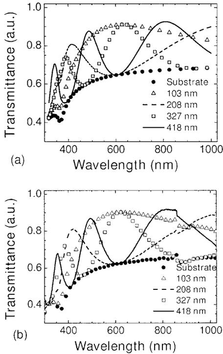
FIG. 1. Transmittance of the  $\text{SiO}_2$  films as a function of wavelength for different film thicknesses: (●) substrate; (△) 103 nm; (---) 208 nm; (□) 327 nm; and (—) 418 nm. (a) Simulated and (b) measured.
