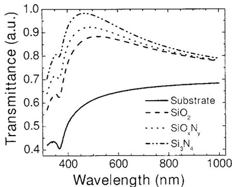
FIG. 5. Optimized transmittances for the  $\text{Si}_3\text{N}_4$ ,  $\text{SiO}_x\text{N}_y$ , and  $\text{SiO}_2$  ARCs as function of the wavelength: (—) substrate; (---)  $\text{SiO}_2$ ; (···)  $\text{SiO}_x\text{N}_y$ ; and (-·-·-)  $\text{Si}_3\text{N}_4$ .
