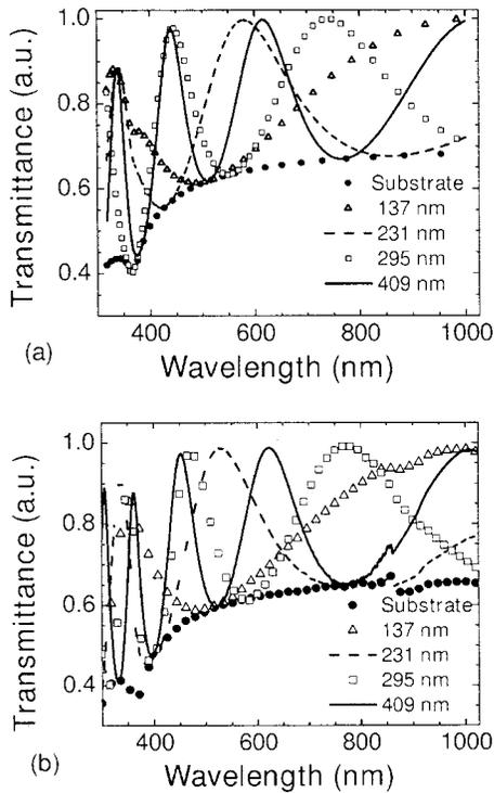
FIG. 2. Transmittance of the  $\text{Si}_3\text{N}_4$  films as a function of wavelength for various thicknesses: (●) substrate; (△) 137 nm; (---) 231 nm; (□) 295 nm; and (—) 409 nm. (a) Simulated and (b) measured.
