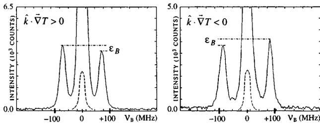
FIG. 2. Experimental spectra for benzene, examples at  $4000\text{ cm}^{-1}$ , with  $|\vec{V}T|=43\text{ K cm}^{-1}$  and  $T=318\text{ K}$  ( $\hat{k}\cdot\vec{V}T>0$ ), and at  $4400\text{ cm}^{-1}$ , with  $|\vec{V}T|=40\text{ K cm}^{-1}$  and  $T=319\text{ K}$  ( $\hat{k}\cdot\vec{V}T<0$ ), respectively. The inset shows the central peak (dotted line), reduced by the factor  $5\times 10^{-2}$ .
