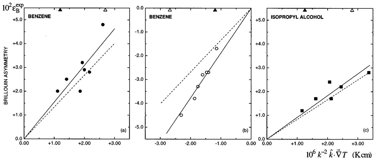
FIG. 3. Measured intensity asymmetry vs a reduced parameter for (a) benzene and (c) isopropyl alcohol, with  $\hat{k}\cdot\vec{V}T>0$ . Data for benzene are again shown in (b), but with  $\hat{k}\cdot\vec{V}T<0$ . Outer open triangles at the top indicate  $4000\text{ cm}^{-1}$ , inner solid triangles  $6000\text{ cm}^{-1}$ , for mean values of  $|\vec{V}T|_m=43\text{ K cm}^{-1}$  for benzene,  $|\vec{V}T|_m=45\text{ K cm}^{-1}$  for isopropyl alcohol.
