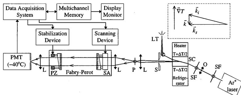
FIG. 1. Schematic diagram of experimental setup and scattering geometry (see inset);  $\vec{k}_i$  is the wave vector of the exciting beam,  $\vec{k}_s$  is the wave vector of the scattered light, and  $\vec{k}$  is the scattering wave vector.
