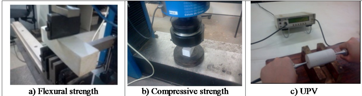
Figure 3: Tests performed: (a) flexural strength, (b) compressive strength, and (c) UPV
