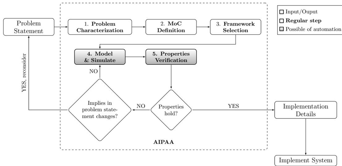
**Figure 2.** Analysis and identification of possible automation approaches (AIPAA) applicable to embedded systems design flow. AIPAA needs the “problem statement” as a given input, and aids to produce a model, which is verified and executable, as output. This output can be used as entry point in the implementation domain, e.g., “implementation details” and “implement system”.
