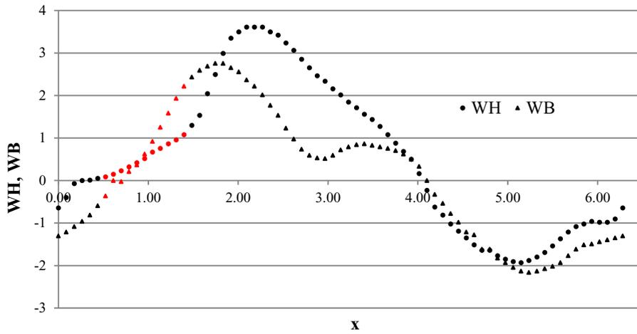
Fig. 1. Head and torque curves in Suter plan.
