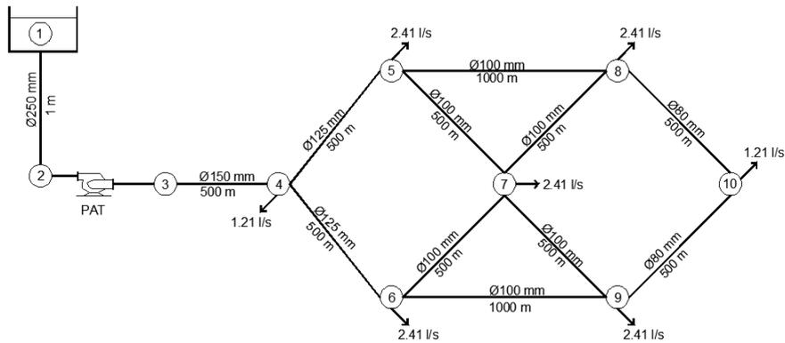
Fig. 3. Layout of water supply network [13].
