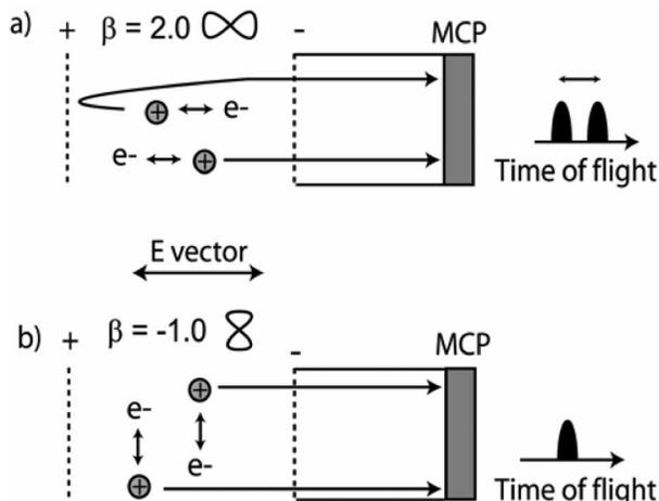
FIG. 2. Effect of the asymmetry parameter  $\beta$  on time-of-flight spectra of cold samples.
