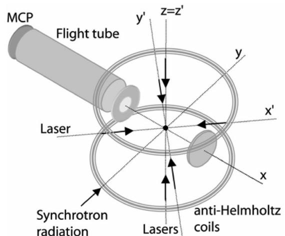
FIG. 1. Schematic view of the experimental setup. The axis of the TOF spectrometer is perpendicular to the propagation direction of the synchrotron UV photons and parallel to their electric field. The six cooling laser beams are located along three orthogonal axis,  $x'$ ,  $y'$ , and  $z'$ . MCP: microchannel plate.
