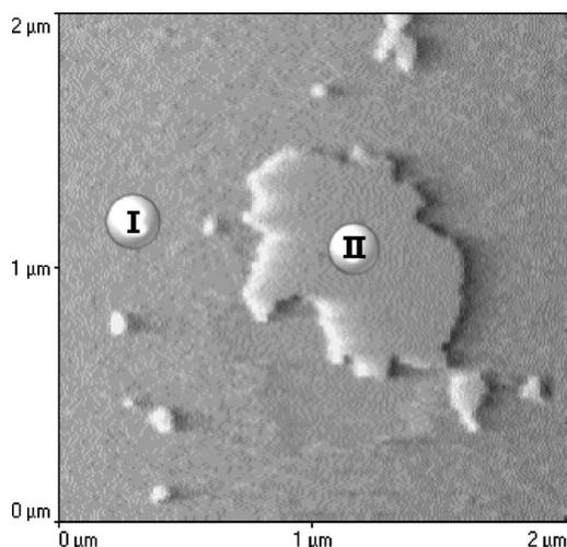
FIG. 1. AFM image of a C<sub>16</sub>TAB adsorbed layer on mica in  $5 \times 10^{-5} M$  C<sub>16</sub>TAB solutions. The islands (patches, region II) indicate higher structures than the background (region I) in agreement with the standard contrast shown by AFM images.
