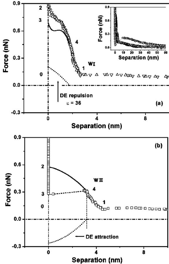
FIG. 2. Force vs separation curves measured for the  $C_{16}TAB$  adsorbed layer on mica in  $5 \times 10^{-5}M$  solutions. (a) Background region and (b) islands. The DEF acting on the tip when immersed in surfactant layer, calculated for a tip with a spherical end with  $R \approx 5$  nm, indicated by the dotted line.
