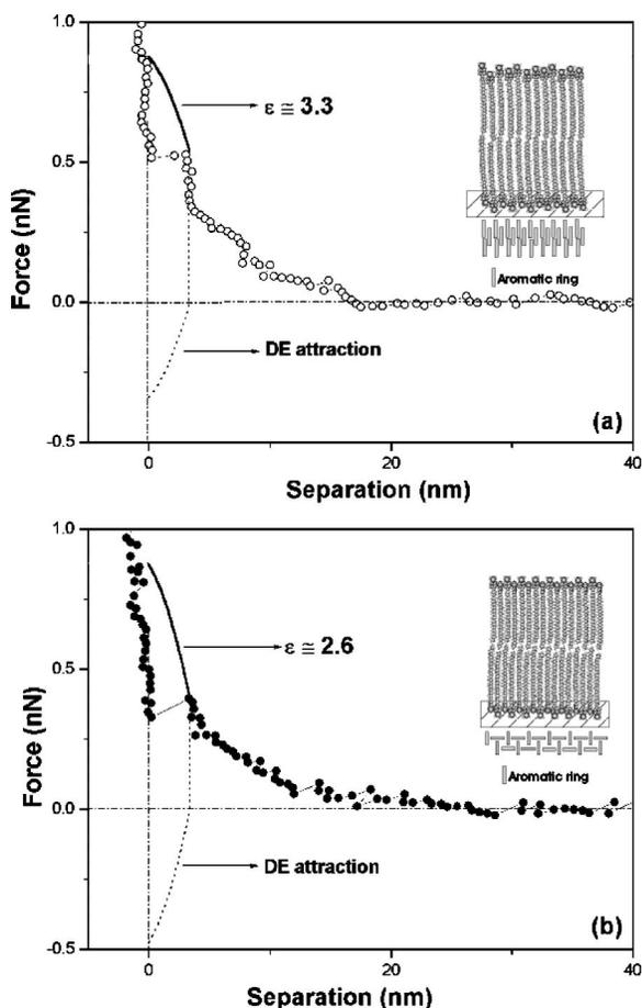
FIG. 6. Force vs separation curve measured in  $5 \times 10^{-3} M$  CPBr solutions. The DEF acting on the tip when immersed in the surfactant layer, calculated for a tip with a spherical end with  $R \approx 5$  nm and using Eq. (1), indicated by the dotted line. (a) for  $\epsilon \approx 3.3$ . Inset: Probable molecular configuration of the CPBr adsorbed layer at the mica interface and (b) the same as in (a) for  $\epsilon \approx 2.6$ .
