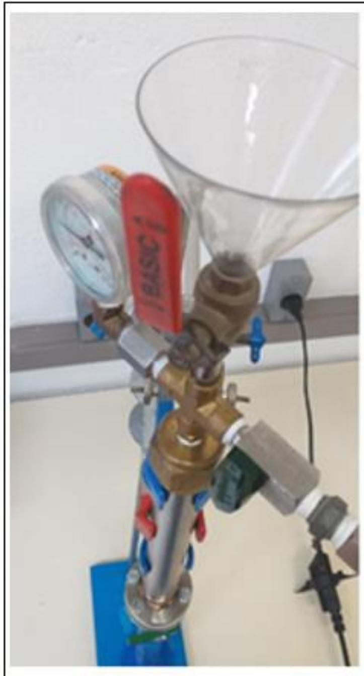
Figure 3.6 – Details of the filter used in microfiltration process (Author, 2021)
