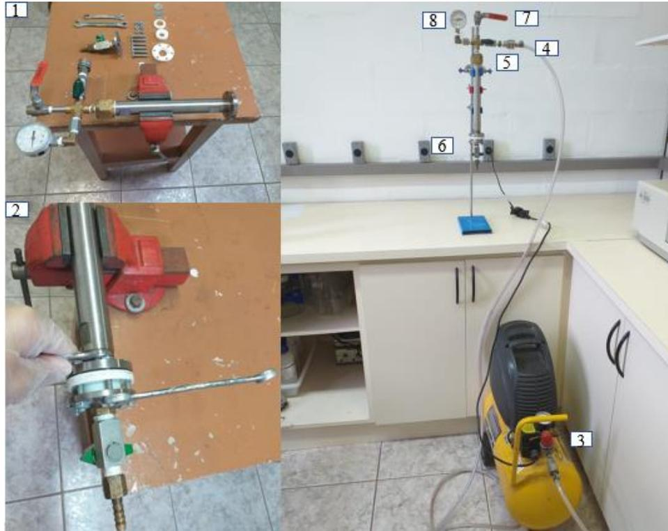
Figure 3.8 - Procedure applied to carry out filtration in a pressurized column (Author, 2021)
