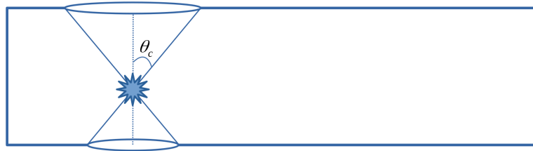
Figure B.1: Solid angle of the photons emitted in the critical angle \theta_C , illustration based on the image found in the MUONCA manual by Prof. Anderson Campos Fauth.
