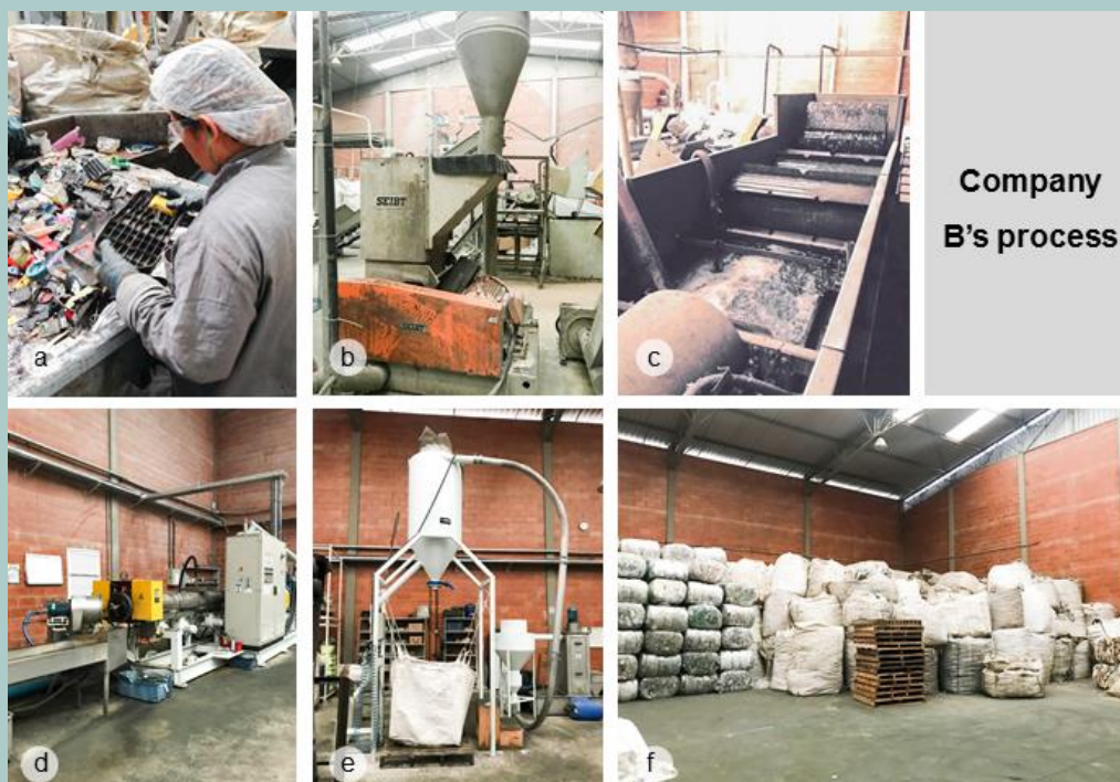
(a) Sorting; (b) Shredding; (c) Washing; (d) Extrusion; (e) Bagging; (f) Stocking Area. Source: Author (2021).
