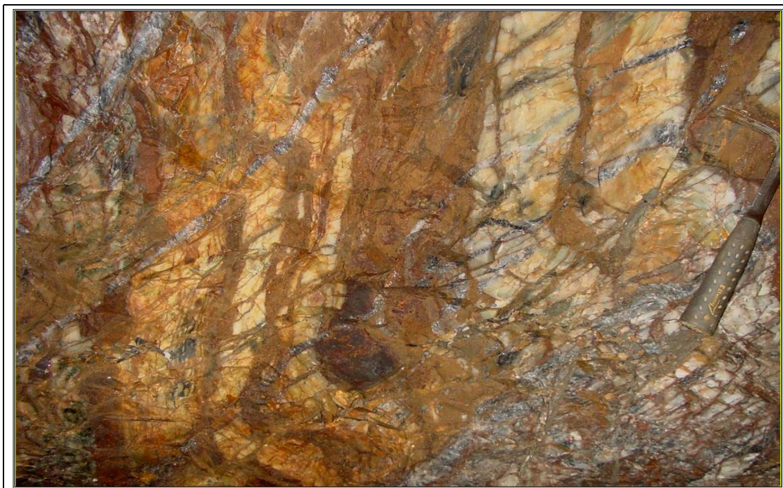
Figure 8 – Banded iron formation (brown portion) with hydrothermal alteration associated, crossed by quartz veins. Cabeça de Pedra orebody.
