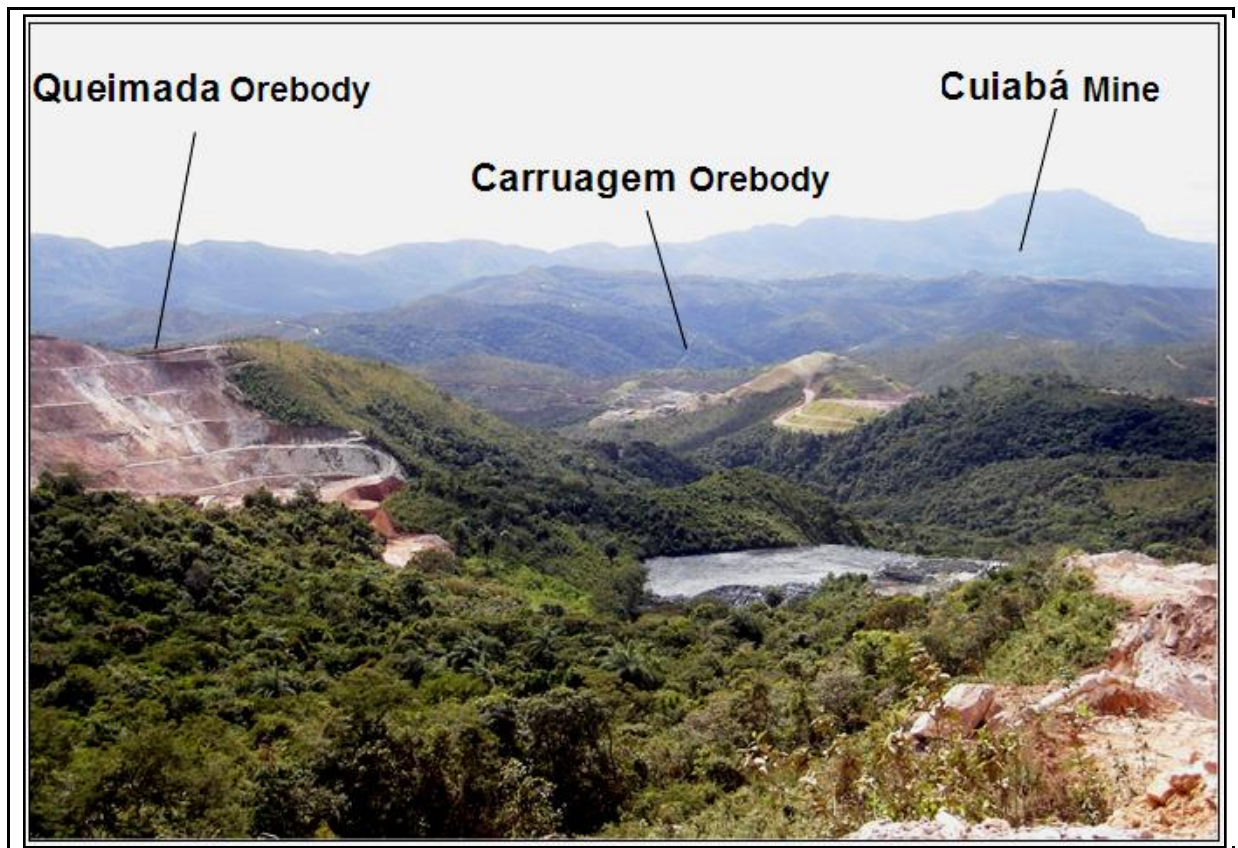
Figure 6 - Wide-angle view of Carruagem and Queimada orebodies (oxidized portion). The large gray patch in the center-right portion of the picture is the waste pile yielded from underground mining operations at the Lamego mine.
