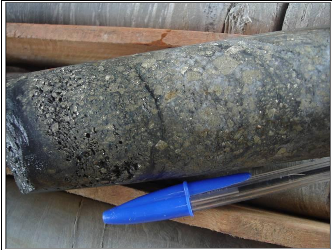
Figure 14 – Drillcore sample with aggregates of pyrites within gray quartz mass.
