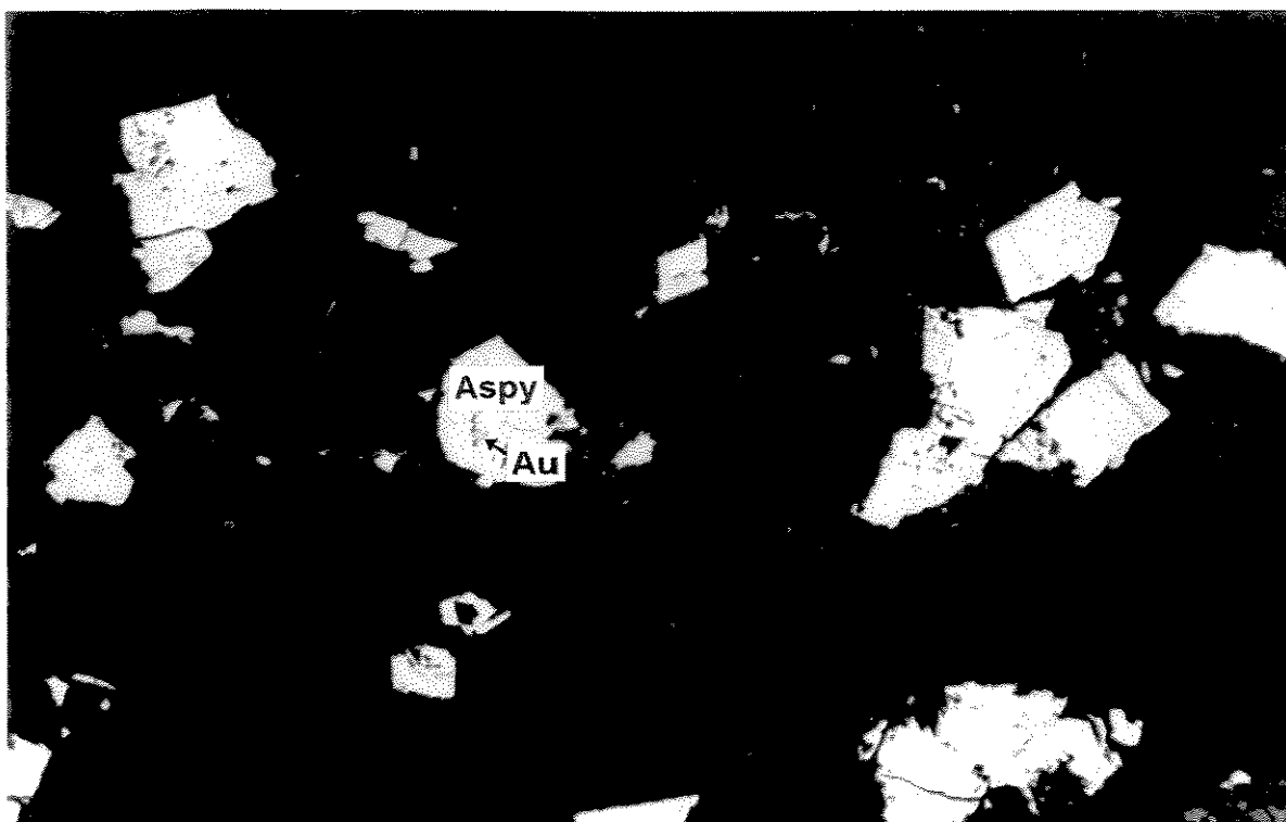
Figure 4.5. Photomicrography showing the mode of occurrence of gold (Au) and its relationship with the main sulfide phases (arsenopyrite - Aspy). Sample GP-115.
