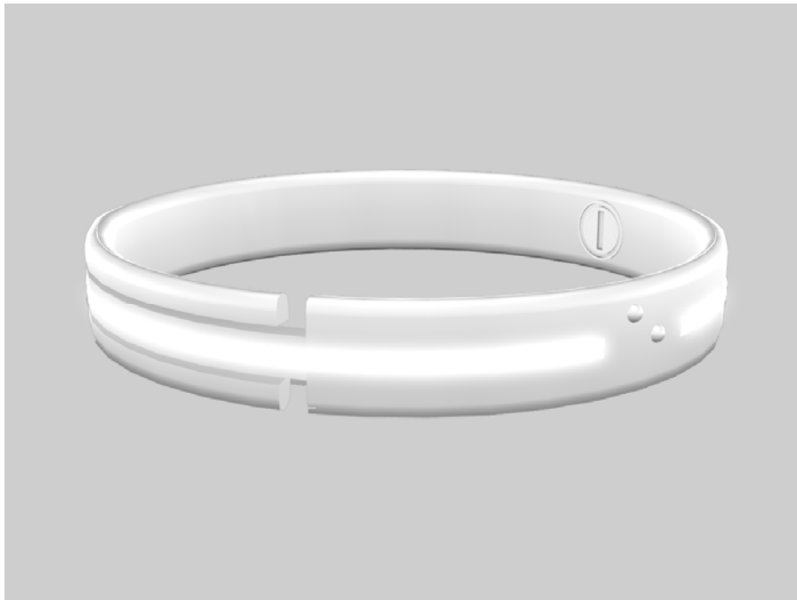
Figure 7.3: AIR with some highlights: Light on, Braille stamp, battery access and mechanical adjustment
