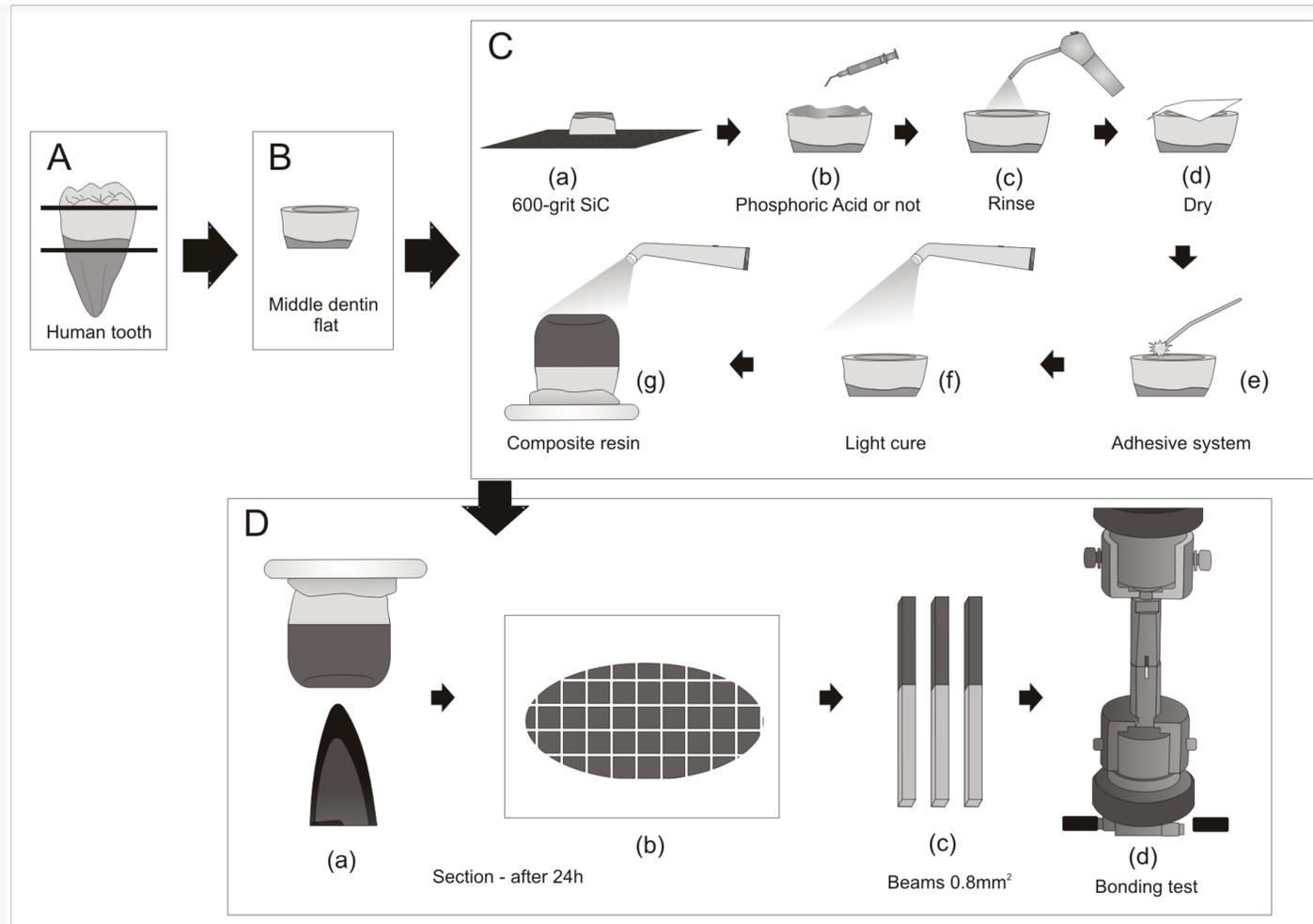
Figure 1. Specimen preparation for microtensile bond strength.
