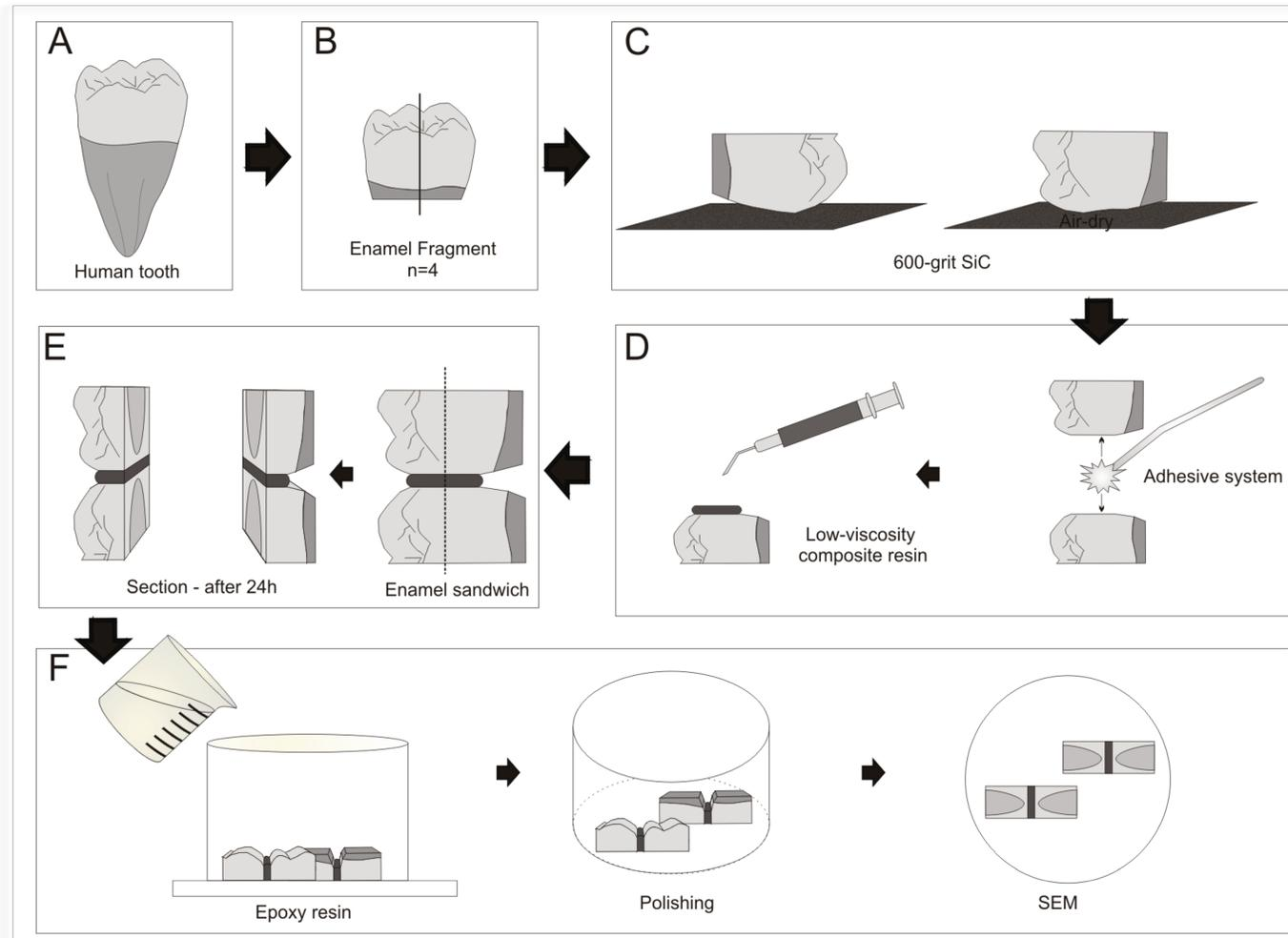
Figure 2. Specimen preparation for interfacial morphology.
