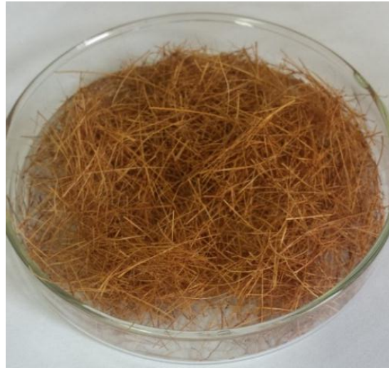
Figura 2.2 Amostra da fibra de coco in natura - \bar{d}_p=359 \mu\text{m}
