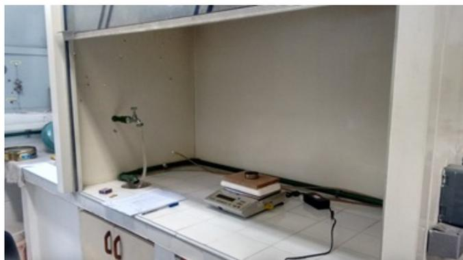
Figure 3.1: Experimental apparatus composed of a scale and a burner inside of a standard fume hood.
